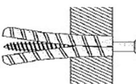
General aerated blocks should not be used to support heavy loads, use a specialist fitting in this case. For light loads, a General Purpose Plug can be used.
