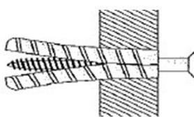
General aerated blocks should not be used to support heavy loads, use a specialist fitting in this case. For light loads, a General Purpose Plug can be used.
